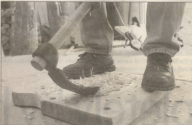
Gerry Felix uses an adze to chip out the depth of the seats. Later, he will use a series of planes and scrapers to form the seat. PHOTO BY DAVE BOWMAN/DAILY PRESS
